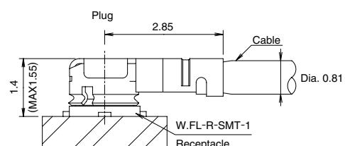
W.FL Series Ultra Small Surface Mount Coaxial Connectors - 1.4mm Mated Height
