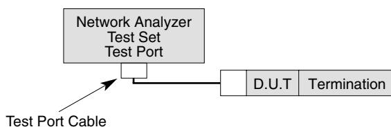
Note1: Measurement way of a W.FL Cable assembly (plug)
