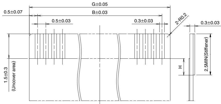
Note 1 : Stiffener dimension should be 2.5mm min., and H dimension should be 0.5mm for improved flexibility of FPC.
